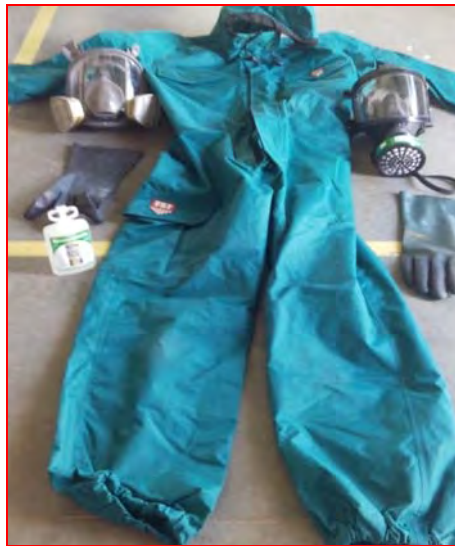
Protective gear that must be available to workers in a Ammonia based refrigeration plant
