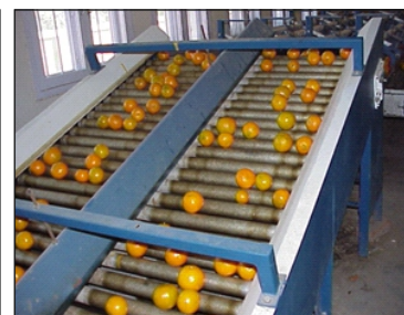
Kinnow washing, grading and waxing lines established by Punjab Agro Industrial Corporation at Hoshiarpur and Abohar
