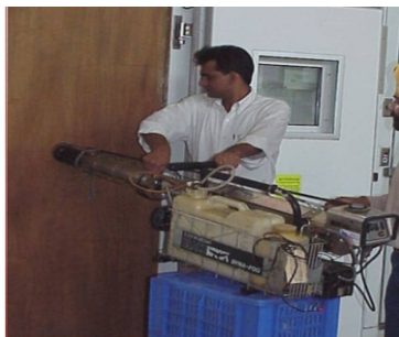
Fig.5. CIPC application with fogging machine
